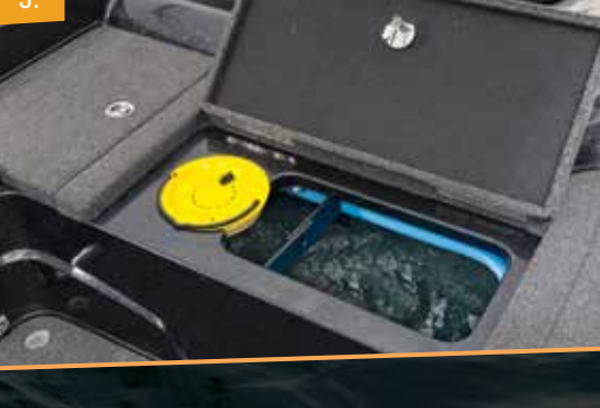
1. Protective dual consoles with high windshields and optional wrap-around walk-thru windshield. 2. 3-level center rod locker with organizers for rods up to 8' (2.44 m) long. 3. Aft 26-gal. (98.42 L) insulated Guardian™ anti-slosh rotomolded livewell with rounded corners, removable divider and bait bucket.
