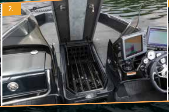
1. Protective dual consoles with high windshields and optional wrap-around walk-thru windshield. 2. 3-level center rod locker with organizers for rods up to 8' (2.44 m) long. 3. Aft 26-gal. (98.42 L) insulated Guardian™ anti-slosh rotomolded livewell with rounded corners, removable divider and bait bucket.
