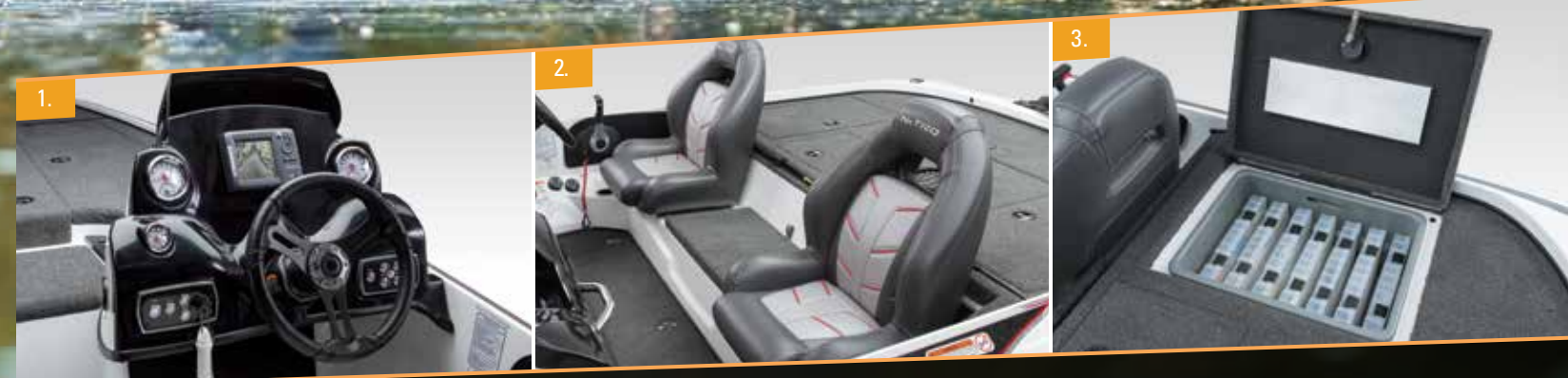
1. There's room for an optional 12" flush-mounted fishfinder on the bow panel and on the driver's console. 2. NASCAR®-inspired seating for all-day comfort on long runs and rough water. 3. 2 aft storage boxes that will each hold seven 3700-style tackle boxes and lift out to allow roomy access to the rigging compartment.
