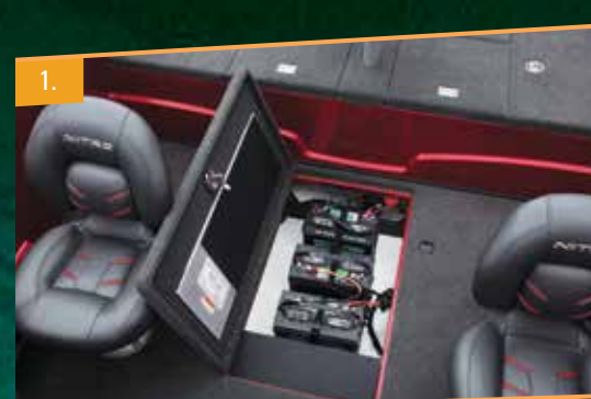
1. Battery storage along keel in center cockpit floor for proper weight distribution and tracking. 2. Driver's side tool organizer and drink holder. 3. 2 aft storage boxes that will each hold seven 3700-style tackle boxes.
