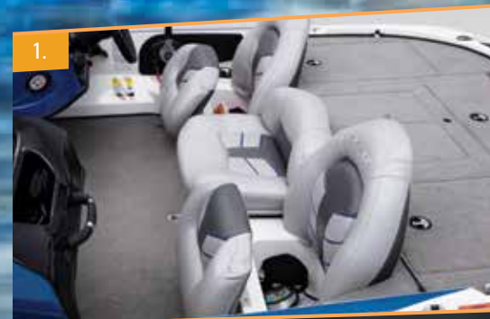
1. Convenient gelcoated storage compartments under driver and passenger seats. 2. Lockable center bow rod storage for rods up to 7'6" (2.3 m). 3. Navigation lights integrated into the gunnels for simple activation.
