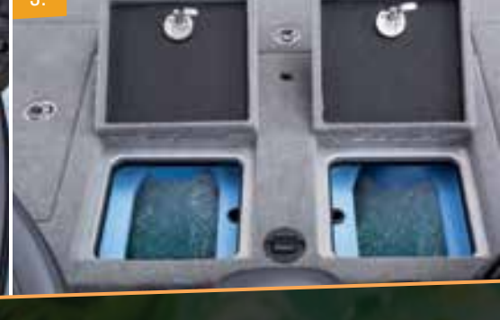
1. Center bow Tackle Management System allows for efficient organization of tackle boxes and bags for quick access. 2. Bow command center with trim, fan and navigation light switches, room for optional 12" flush-mount fishfinder and tool/drink holder. 3. 2 NITRO®-exclusive 19-gal. (71.92 L) Guardian™ livewells with anti-slosh lip, freshwater pump, recirculator, timers and pump-out.
