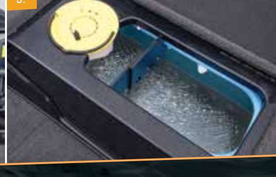
1. Protective dual consoles with high windshields and optional wrap-around walk-thru windshield. 2. 3-level center rod locker with organizers for rods up to 8' (2.44 m) long. 3. Aft 26-gal. (98.42 L) insulated Guardian™ anti-slosh rotomolded livewell with rounded corners, removable divider and bait bucket.
