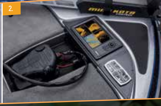
1. Center bow Tackle Management System allows for efficient organization of tackle boxes and bags for quick access. 2. Bow command center with trim, fan and navigation light switches, room for optional 12" flush-mount fishfinder and tool/drink holder. 3. 2 NITRO®-exclusive 19-gal. (71.92 L) Guardian™ livewells with anti-slosh lip, freshwater pump, recirculator, timers and pump-out.
