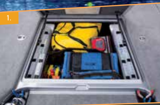
1. Center bow Tackle Management System allows for efficient organization of tackle boxes and bags for quick access. 2. Bow command center with trim, fan and navigation light switches, room for optional 12" flush-mount fishfinder and tool/drink holder. 3. 2 NITRO®-exclusive 19-gal. (71.92 L) Guardian™ livewells with anti-slosh lip, freshwater pump, recirculator, timers and pump-out.
